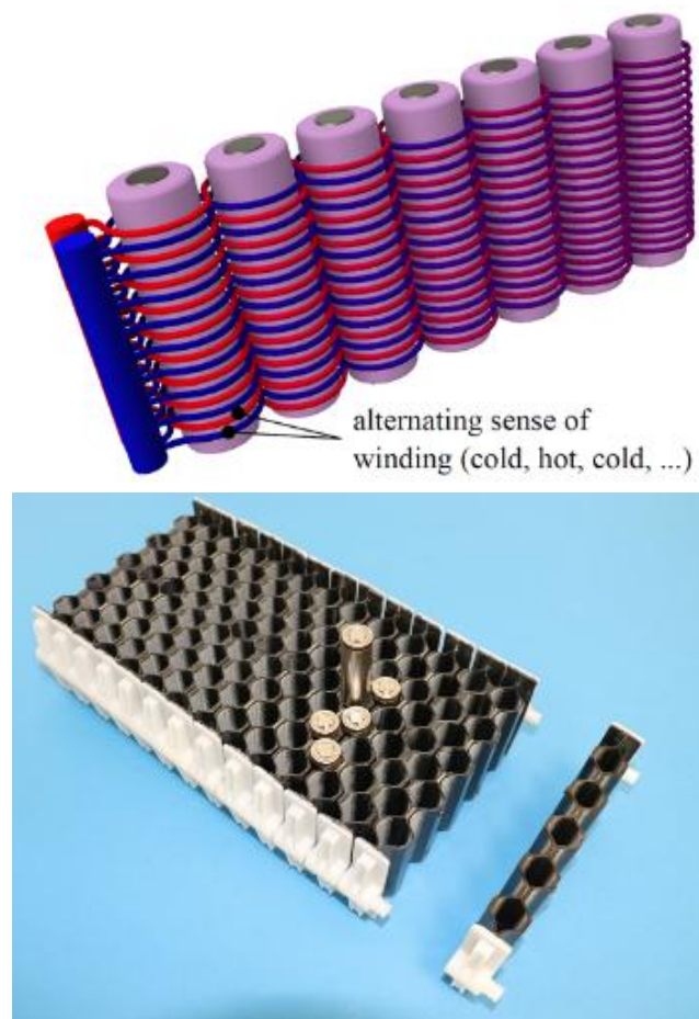
Fig. 6 Cooling of cylindrical electrical cells, on the right is the block for the cell set
